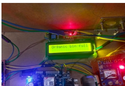
Fig.4: Display bin levels in LED
