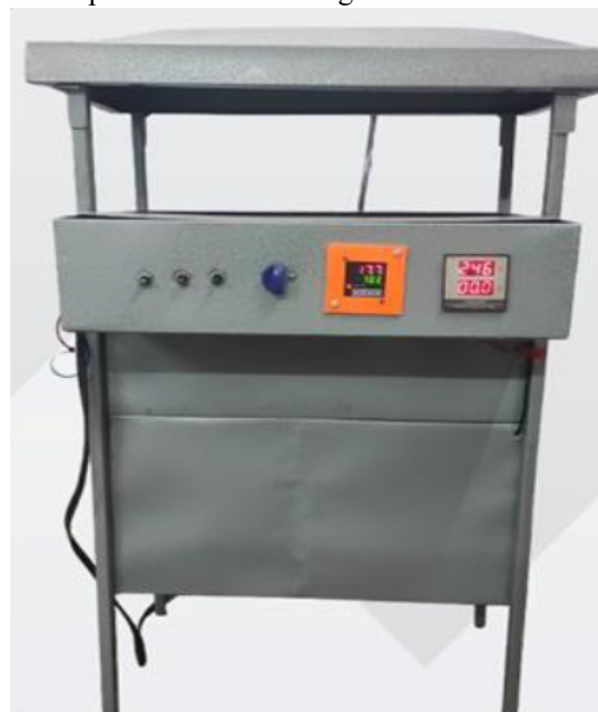
Figure 2. Photograph of the developed RWD showing the drying unit and integrated temperature-control panel.
